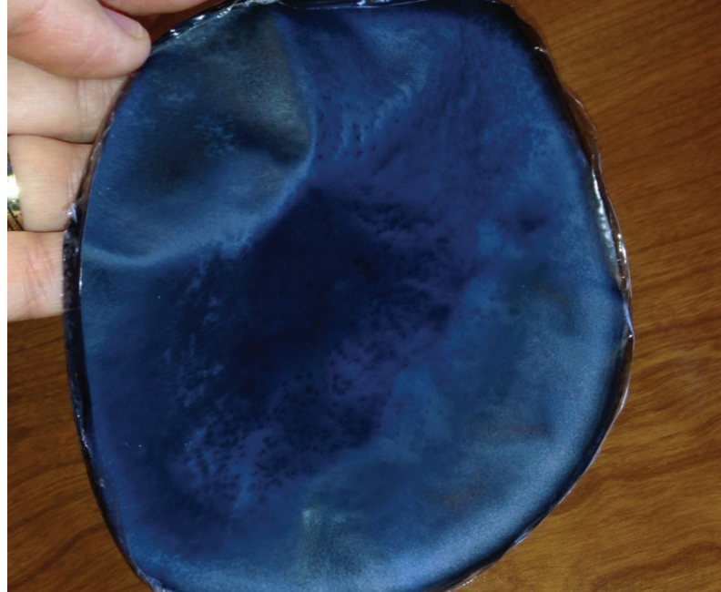
Film prepared from chicken feather keratin. Black powder was added to film formulation as a filler for effective sunlight absorption.
