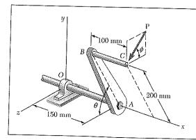
A single force **P** acts at *C* in a direction perpendicular to the handle *BC* of the crank shown. Knowing that  $M_x = +20 \text{ N} \cdot \text{m}$  and  $M_y = -8.75 \text{ N} \cdot \text{m}$ , and  $M_z = -30 \text{ N} \cdot \text{m}$ , determine the magnitude of **P** and the values of  $\phi$  and  $\theta$ .
