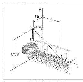
A small boat hangs from two davits, one of which is shown in the figure. It is known that the moment about the z-axis of the resultant force  $\mathbf{R}_A$  exerted on the davit at A must not exceed 279 lb·ft in absolute value. Determine the largest allowable tension in line ABAD when x = 6 ft.
