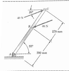
Two parallel 40-N forces are applied to a lever as shown. Determine the moment of the couple formed by the two forces (a) by resolving each force into horizontal and vertical components and adding the moments of the two resulting couples, (b) by using the perpendicular distance between the two forces, (c) by summing the moments of the two forces about Point A.
