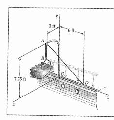
A small boat hangs from two davits, one of which is shown in the figure. The tension in line ABAD is 82 lb. Determine the moment about C of the resultant force  $\mathbf{R}_A$  exerted on the davit at A.
