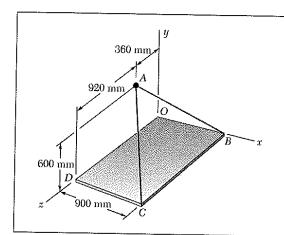
Knowing that the tension in cable AB is 570 N, determine the moment about each of the coordinate axes of the force exerted on the plate at B.
