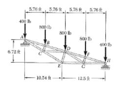
4. A Warren bridge truss is loaded as shown. Determine the force in members *EG*, *FG*, and *FH*.
