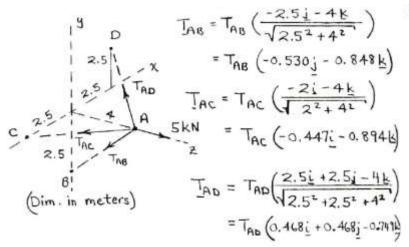
$$\begin{split} \sum F_{X} = 0: & -0.447 \, T_{AC} + 0.469 \, T_{AD} = 0 \\ \sum F_{Y} = 0: & -0.530 \, T_{AB} + 0.469 \, T_{AD} = 0 \\ \sum F_{Z} = 0: & -0.848 \, T_{AB} - 0.874 \, T_{AC} - 0.749 \, T_{AO} + 5 = 0 \\ \text{Solution:} \quad \underbrace{T_{AB} = 1.814 \, kN}_{T_{AC}}, \quad \underbrace{T_{AC} = 2.15 \, kN}_{T_{AD}} \end{split}$$
