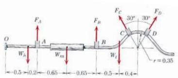
Solution: For a zero force - couple system at point 0:
