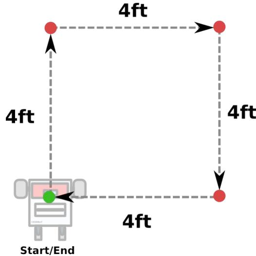
2. Measure how well your 'odometry' performs. Recall that your robot relies on 'relative' odometry assumptions to determine how far it has traveled, and how far it has turned. If odometry readings are perfect, then the robot should make a perfect square. Therefore perform the following:
