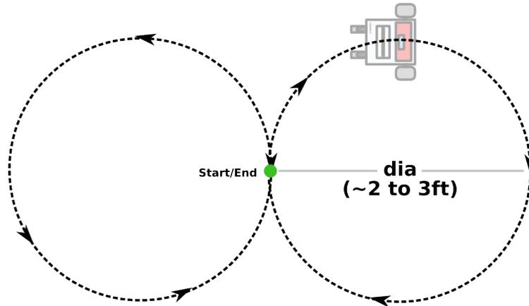
**Note:** This is not as easy as it sounds. You need to look at the *Programmer's Reference* manual for the API and determine which functions will empower to you achieve this goal. For example, maybe you'll need to issue a command in *free-running* mode and then 'modulate' the speed of left and right motors accordingly to achieve the figure-eight pattern. As a tip – look at `STEPPER_run()` and `STEPPER_set_speed()` functions.
