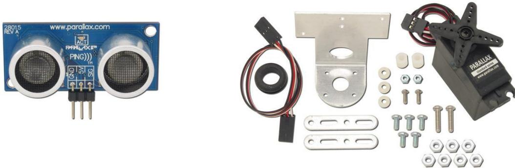
For this laboratory exercise you will be using the *Parallax PING))) Ultrasonic Distance Sensor* (#28015 – pictured above on the left) and will assemble and attach it using the mounting bracket and screws onto the RC servo (pictured above on the right) in preparation for future upcoming labs. For *this* laboratory exercise, however, you will focus only on assembling the unit, and using the ultrasonic sensor alone, mounted on the CEENBoT so that it faces forward.
