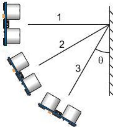
3. Next, position your CEENBoT 12 inches from the wall at 90-degrees as shown in the previous figure. Record the distance detected. Then, move the CEENBoT at smaller angles (as shown (2) and in (3) in the previous figure) from the wall. Each time, record the distance detected. Do the values change? At what angle does the sensor cease to detect the wall?
