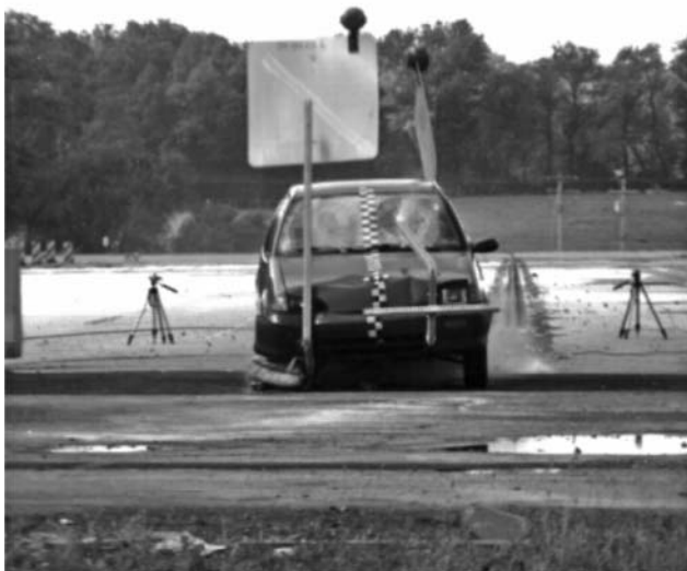
Figure 6. H-base sign panel separation due to vehicle impact.
