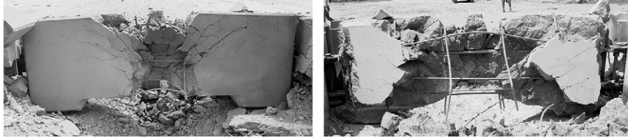
Fig. 4. Control (K-1) barrier after test: front (left) and back (right).
