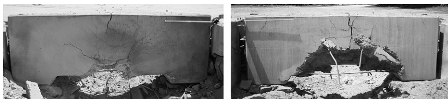
Fig. 6. Nylon fiber (NFRC) barrier after test: front (left) and back (right).
