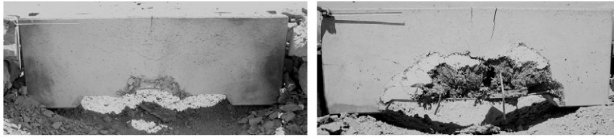
Fig. 7. Low volume steel/synthetic fiber (SS-L) barrier after test: front (left) and back (right).
