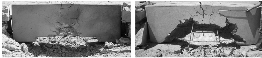
Fig. 5. Carbon fiber barrier (CFRC) barrier after test: front (left) and back (right).
