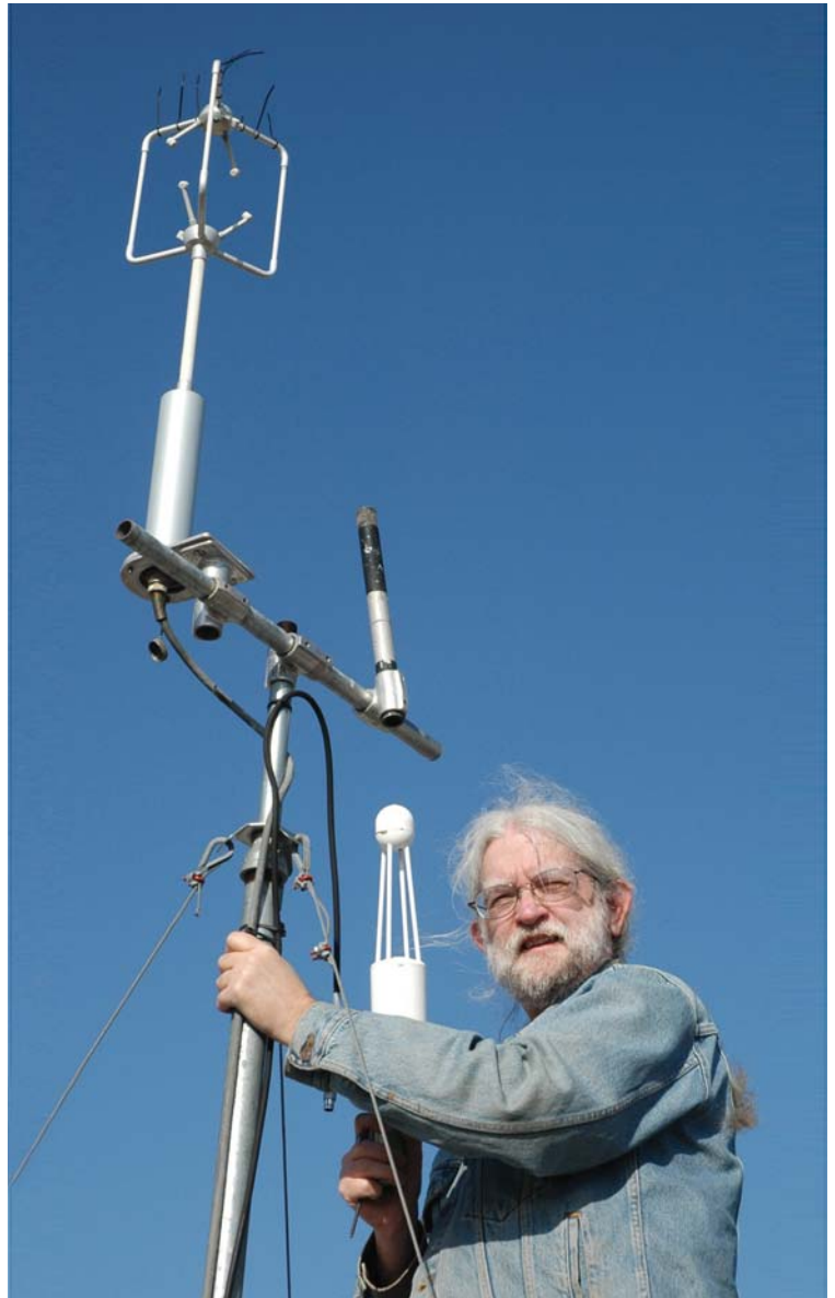
Department physicist, Dr. David Billesbach , monitors a weather station at the UNL Gudmundsen Sandhills Laboratory. Used to collect data concerning water balance (rain in/water vapor out), these stations are set up for long-term research on how the prairie grass cover interacts with the aquifer. This grass is the underpinning for the Sandhills cattle industry. Photo used with permission.
