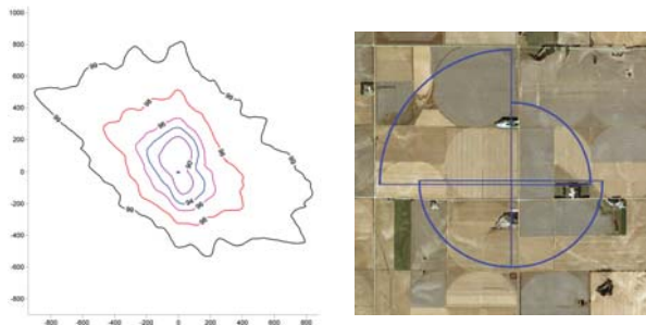
On the left is an example output from the odor modeling. This output is then converted into the OFT setback distances (on the right) by taking the longest distance in each sector to give an easy-to-visualize footprint for the odor drift from a livestock operation. The blue lines represent the minimum separation distance for a specific odor tolerance level.
