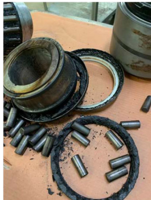
Figure 8. Results from the accelerated life test: (a) IB inner ring assembly, (b) IB inner ring assembly removed from the bearing
