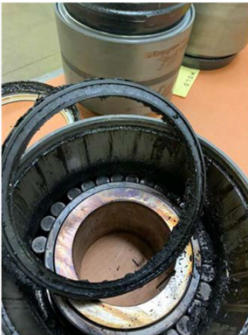
Figure 8. Results from the accelerated life test: (a) IB inner ring assembly, (b) IB inner ring assembly removed from the bearing
