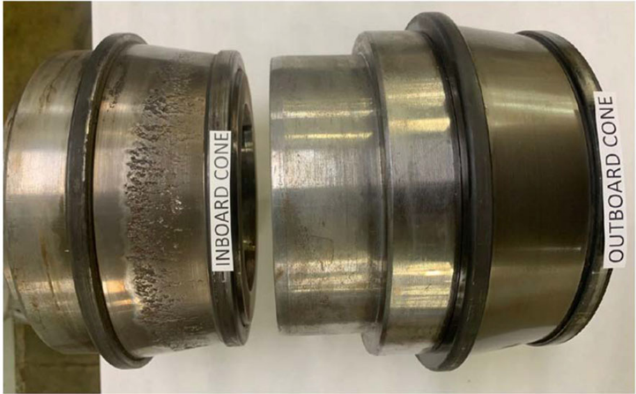
Figure 9. Results from the accelerated life test: IB and OB inner ring raceways.
