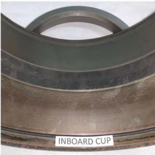
Figure 10. Results from the accelerated life test: (a) IB outer ring raceway, (b) OB outer ring raceway
