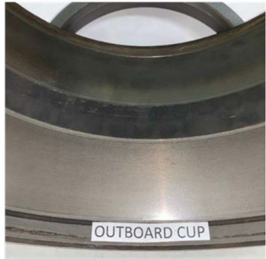
Figure 10. Results from the accelerated life test: (a) IB outer ring raceway, (b) OB outer ring raceway
