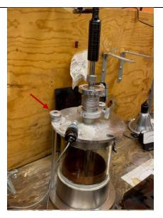
7. Turn on the pump(turning counterclockwise and the pressure gage should go down, means the system is working) then for accelerating the process do the 5-6 pump and flush cycles( replacing the atmosphere with Argon gas). During pumping and flushing check the pressure on the pressure gage. It must become under 100 Mtorr.
