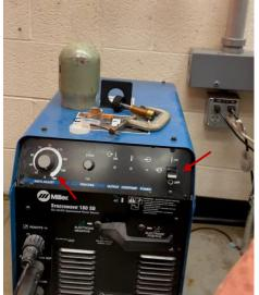
11. Put the shield glasses. Put the electrode tip in the middle on the copper and start pressing the pedal slowly to see the lights.
