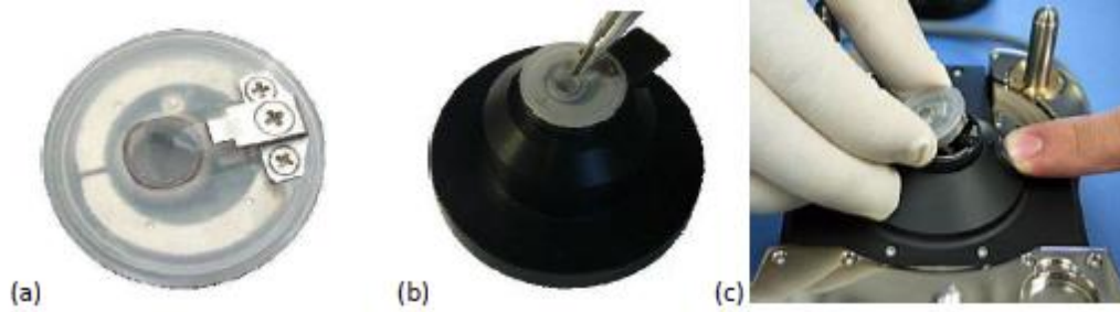
Figure 2: (a) AFM tip holder assembly; (b) holder assembly in the loading pedestal; (c) Removing tip holder assembly from AFM head.
