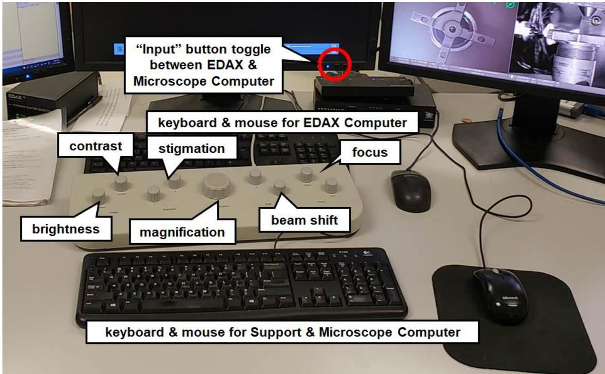
Figure 9: Helios 660 control panel
