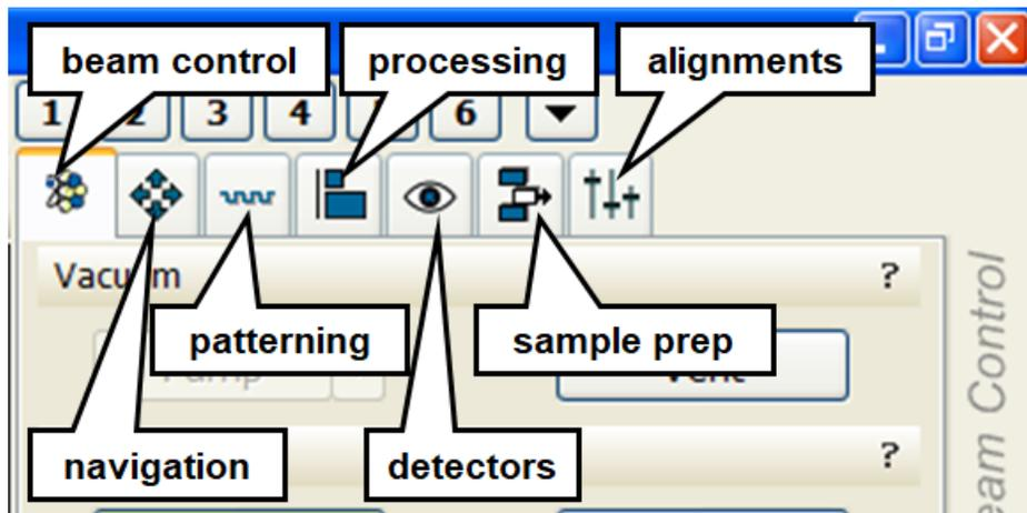
Figure 5: Microscope Control Program Tabs
