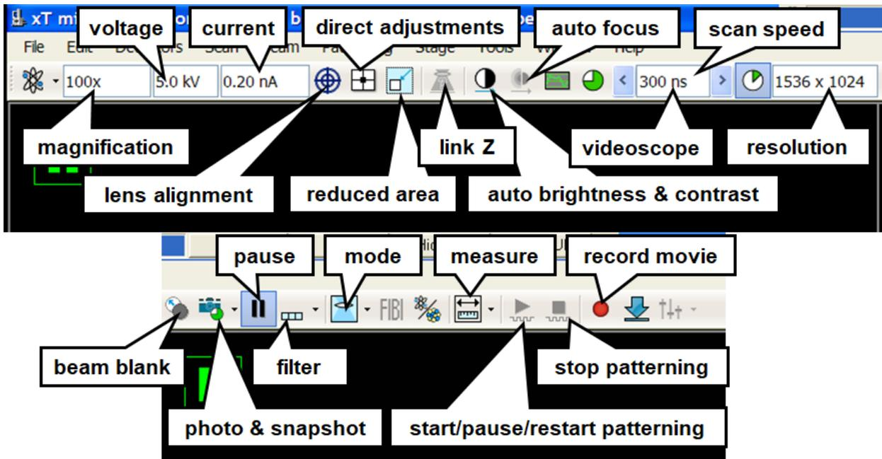
Figure 4: Microscope Control Program Toolbar
