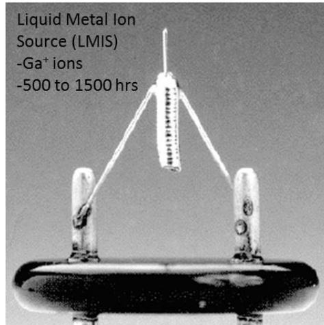
**Figure 11: Ga Ion Source for the FIB**
