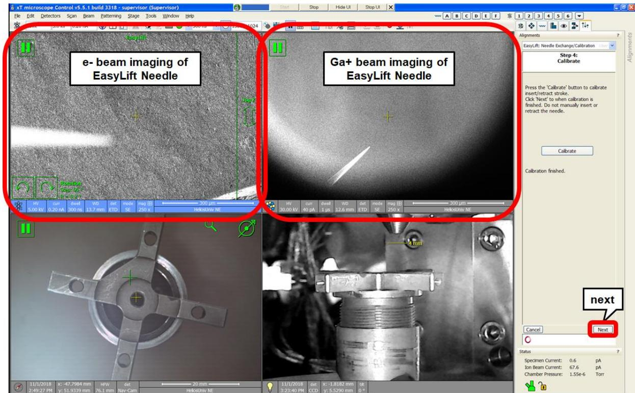
**Figure 17: Step 4 After Insert Needle**
