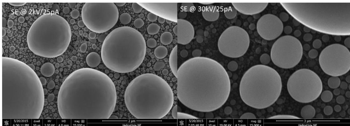
**Figure 10: SEM secondary electron images taken with Mode 1 and 2.**
