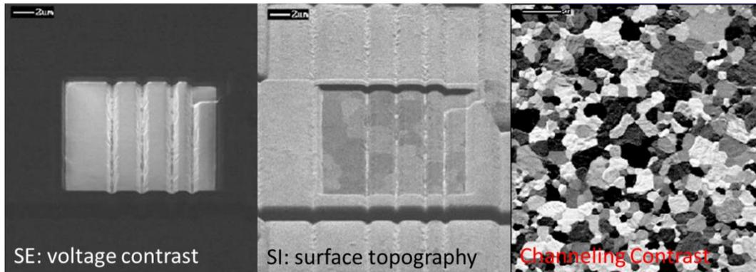
**Figure 13: Comparison of SEM voltage, topographical, and channeling contrasts**
