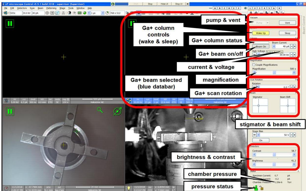
Figure 12: Beam Control Tab for Ion Beam (Note: it's completely different from Electron Beam)
