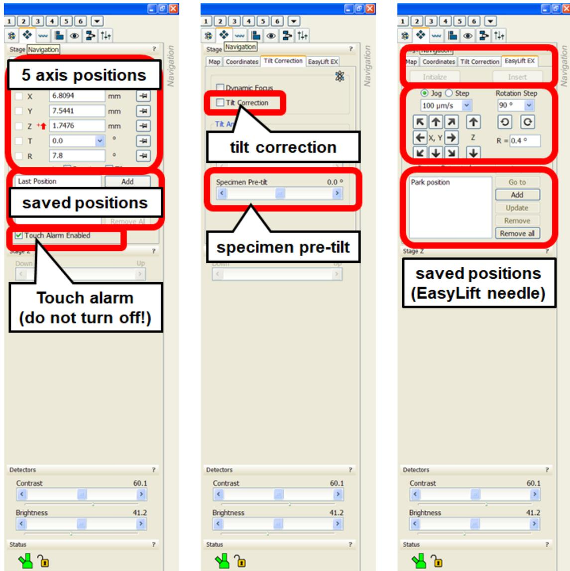
Figure 7: Navigation Tab with Coordinates, Tilt Correction, and EasyLift
