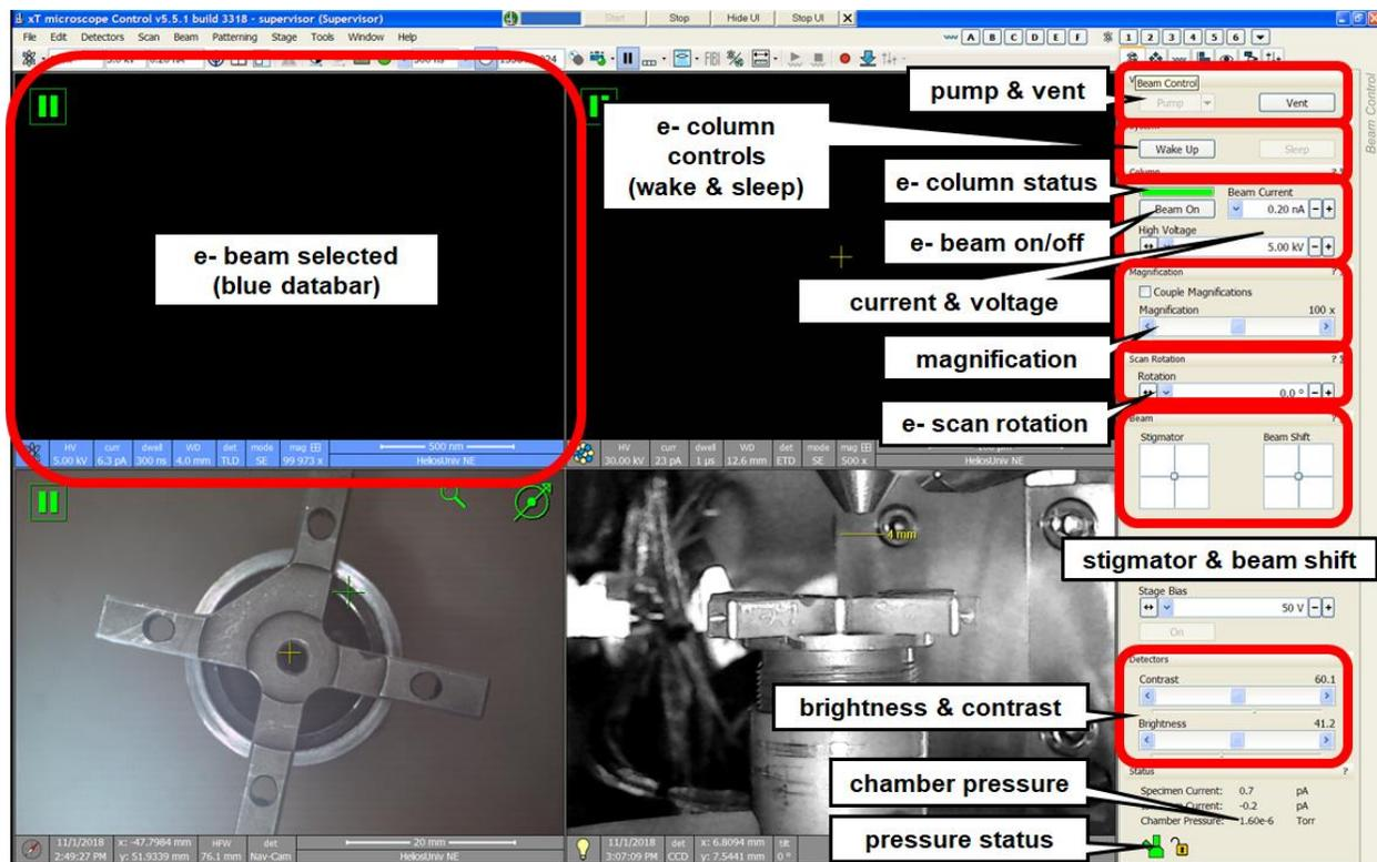
**Figure 8: Beam Control Tab for Electron Beam (Note: it's completely different from Ion Beam)**
