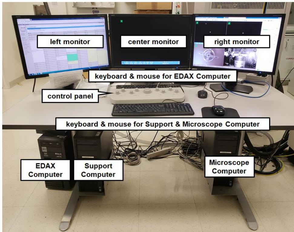
**Figure 2: Helios 660 computers and control panel**
