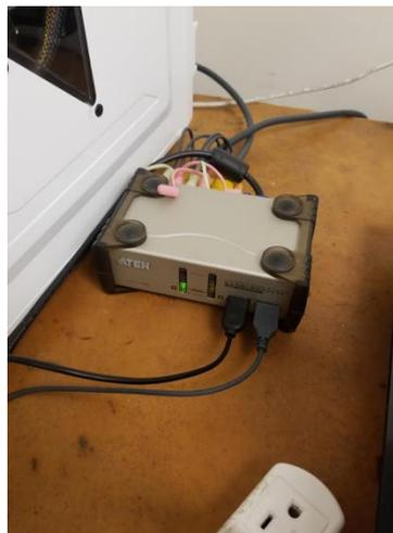
Figure 7: MASTER VIEW KVMP SWITCH box
