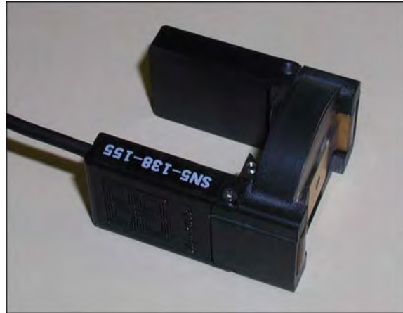
Figure 1.14 Transducer ready for probe installation
