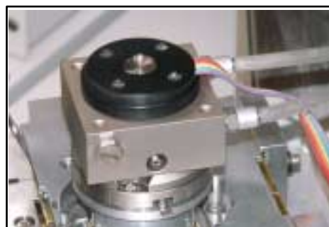
FIGURE 9-18 COLD STAGE INSTALLED
