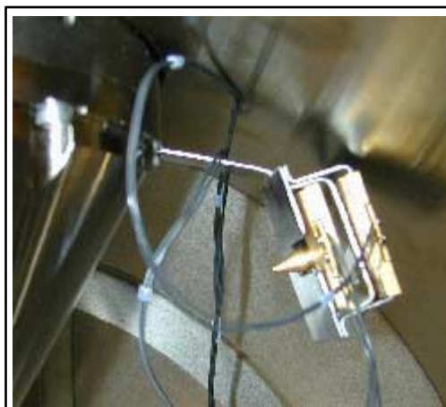
FIGURE 9-8 HOME POSITION FOR GAD AND BSD
