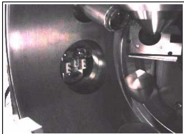
FIGURE 9-51 CHAMBER FEEDTHROUGH (INSIDE)
