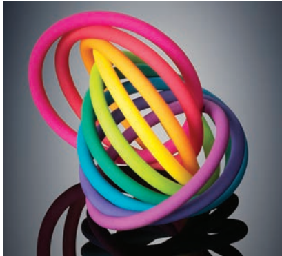
Figure 3: These interlocking color rings were 3D printed in one job using the cyan-magenta-yellow palette.
