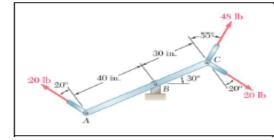
Three control rods attached to a lever ABC exert on it the forces shown. (a) Replace the three forces with an equivalent force-couple system at B. (b) Determine the single force that is equivalent to the force-couple system obtained in Part a, and specify its point of application on the lever.
