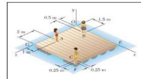
Three children are standing on a  $5 \times 5$ -m raft. If the weights of the children at Points A, B, and C are 375 N, 260 N, and 400 N, respectively, determine the magnitude and the point of application of the resultant of the three weights.
