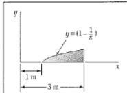
Locate the centroid of the volume obtained by rotating the shaded area about the x-axis.
