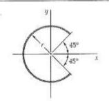
A homogeneous wire is bent into the shape shown. Determine by direct integration the x coordinate of its centroid.
