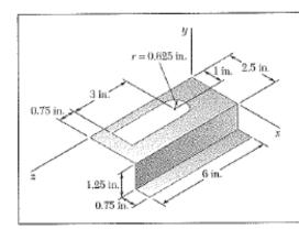
A mounting bracket for electronic components is formed from sheet metal of uniform thickness. Locate the center of gravity of the bracket.
