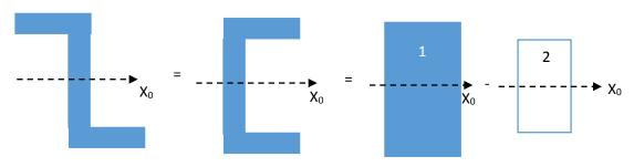
$$I_{x_0} = I_{1x_0} - I_{2x_0} = \frac{1}{12} \left[ bh^3 - b'^{h'^3} \right] = \frac{1}{12} \left[ 100 * 160^3 \ mm^4 - 80 * 120^3 \ mm^4 \right] = 22,613,333 \ mm^4$$
