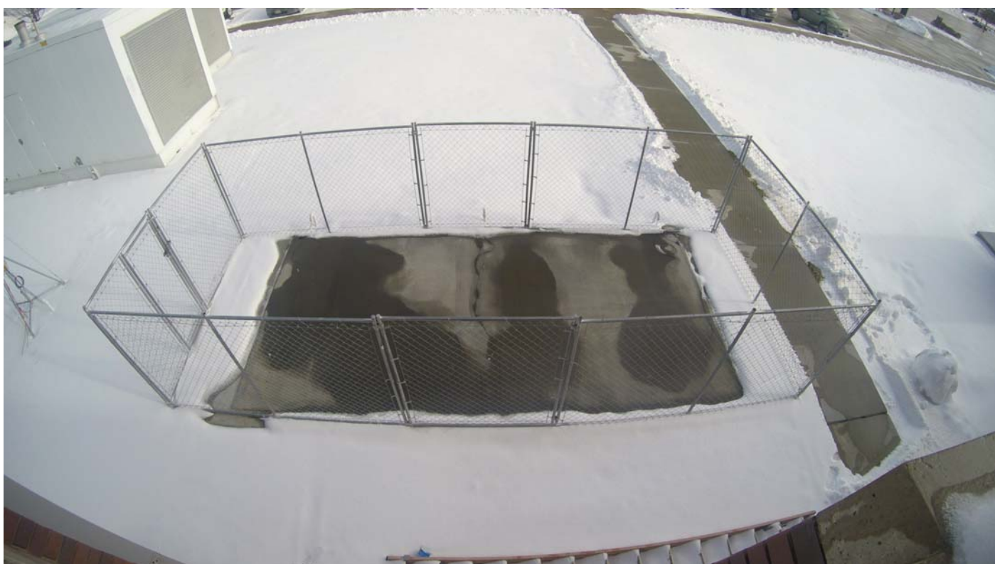
Figure 4: Heated test pad after the snowstorm on 27–28 December 2015.
