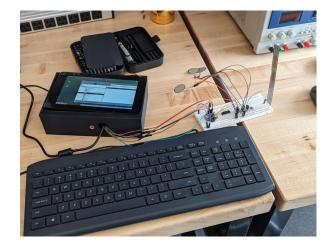
Hand and wrist repetitive stress injuries are common among sonography staff. These injuries are caused by excessive grip pressure exerted on the probe for long periods of time. Our team was tasked with developing a system to track sonography students' grip pressure and provide alerts when excessive grip pressure is used. The goal is to use this feedback system to help develop healthy muscle memory for the grip used by ultrasound operators.
