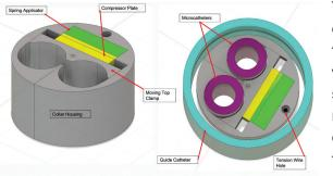
This device will be used for intravascular catheterization procedures, specifically the treatment of intracranial aneurysms. The device will allow for two microcatheters to be used simultaneously with the ability to limit their motion relative to one another. The goal of this device is to give physicians more flexibility in the treatment of intracranial aneurysms.
